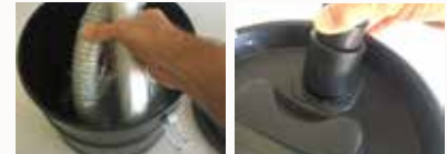
Release lid and remove all contents from inside canister. Insert included pickup hose into receiver on lid. Line up pin so it will drop in slot.
