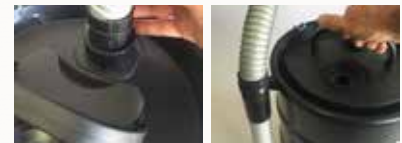
Twist hose to lock into lid. Put nozzle on hose end and attach to side of canister.
