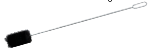
ITEM #: 2707 4" diameter x 6" tall soft bristle brush. For hand working straight sections of 4" vents. Twisted wire stem is quite rigid. 42" overall length.
