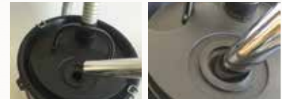
Insert household vacuum tube into rubber grommet. Rubber expands to seal most vacuum hoses. If seal does not fit try another vacuum.
